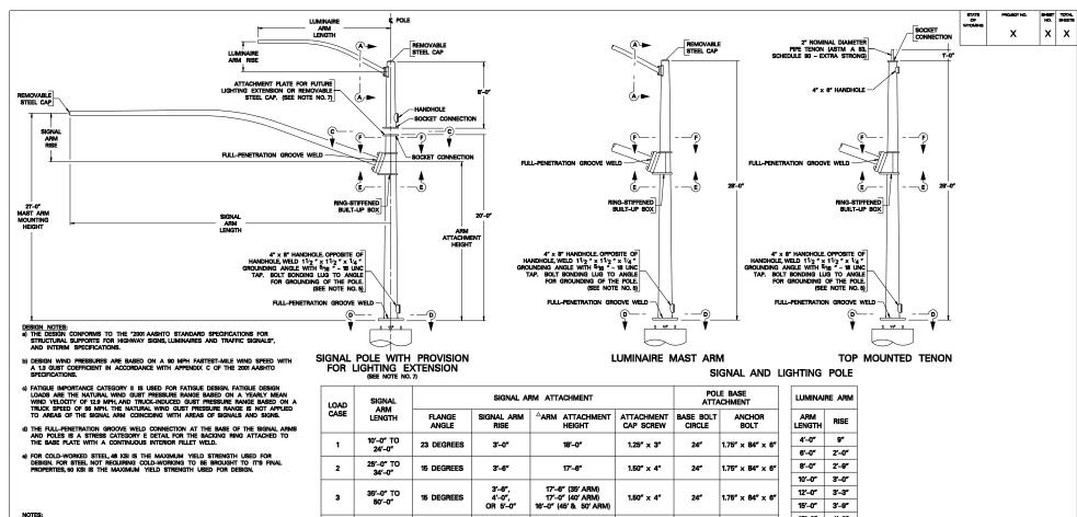
1. USE ANCHOR BOLTS CONFORMING TO AASHTO M 314 WITH A YIELD STRENGTH OF 55 KSI. SUPPLY TWO NUTS AND TWO WASHERS WITH EACH ANCHOR BOLT.
