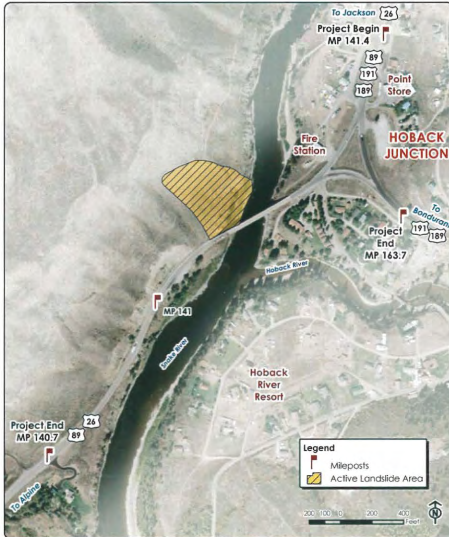
Figure 1-6 Active Landslide Area
