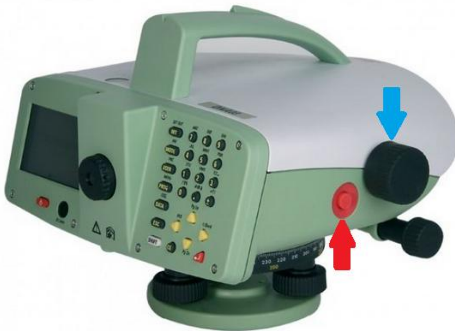
Figure 9-21. Focus knob and measure button.
