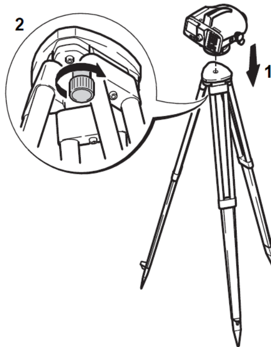
Figure 9-1. Instrument and tripod setup.
