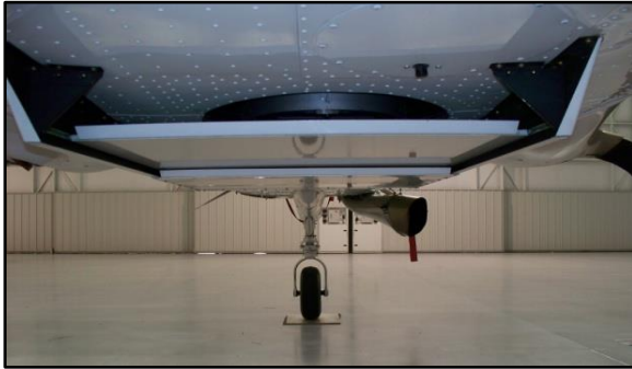
Image VII-2. Sliding door for lens protection
