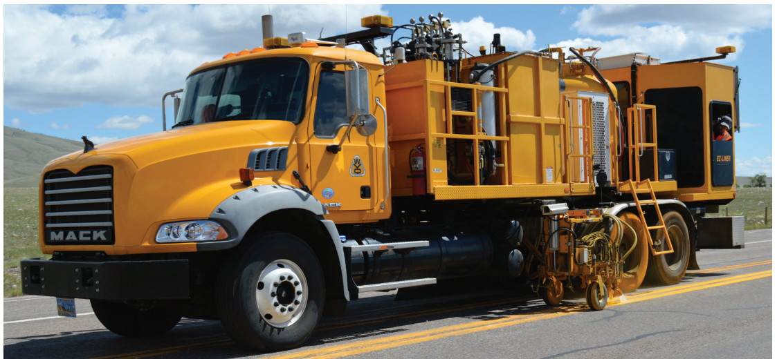
A WYDOT striping vehicle applying fresh paint during spring highway striping operations.
