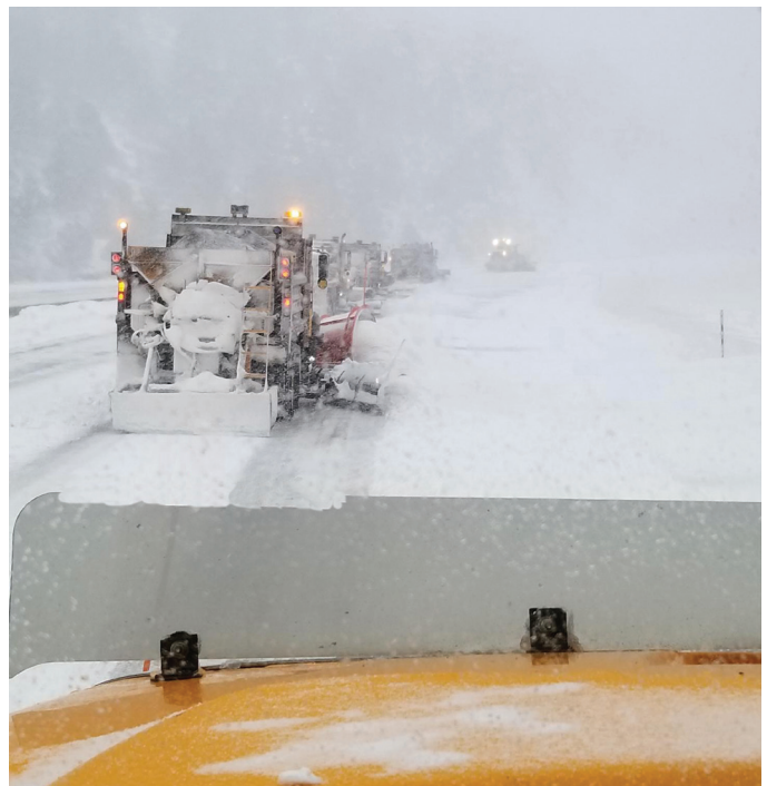
A snow maintainer's view from the cab of a plow truck clearing snow from multiple lanes at once.
