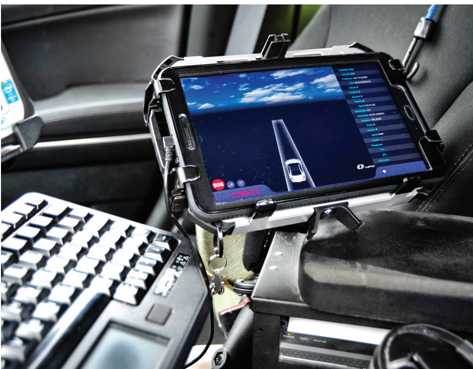
In-cab equipment needed for WYDOT's Connected Vehicle Pilot.
