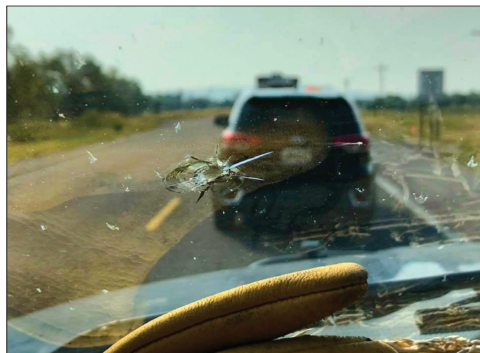
Fresh chip sealing can create the risk of flying rock at unsuspecting drivers and windshields.
