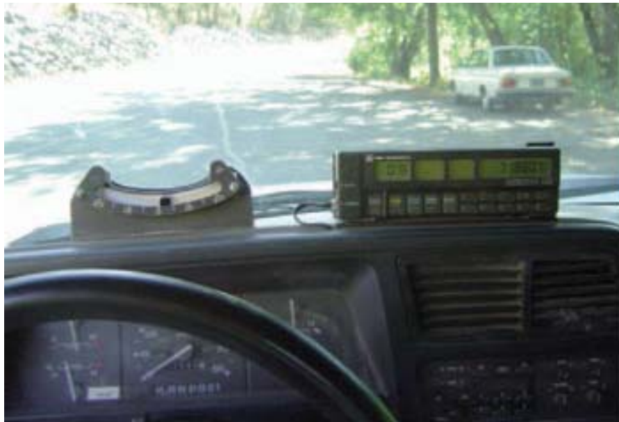
Figure 11-2 Example of Equipment Used for the Ball-bank Indicator Method
