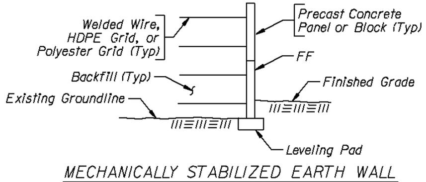
**EMBANKMENT REINFORCEMENT SYSTEMS** are geotextiles or welded wire reinforcement mats placed in single layers that mechanically interlock with the material being reinforced. The layers can be wrapped to the next layer of backfill at the face of the embankment to form a sloped surface or the layers can be attached to blocks to form a wall.
