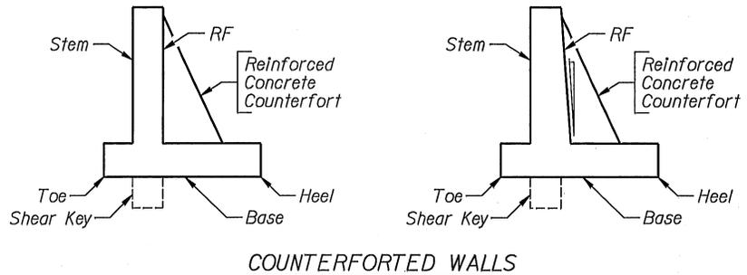
**EXPANSION JOINTS** and **CONTRACTION JOINTS** may be required for cantilever and counterforted walls. Expansion joints shall be provided if the wall length exceeds 90'-0". Contraction joints shall be provided at spacings of 20'-0" minimum to 30'-0" maximum.
