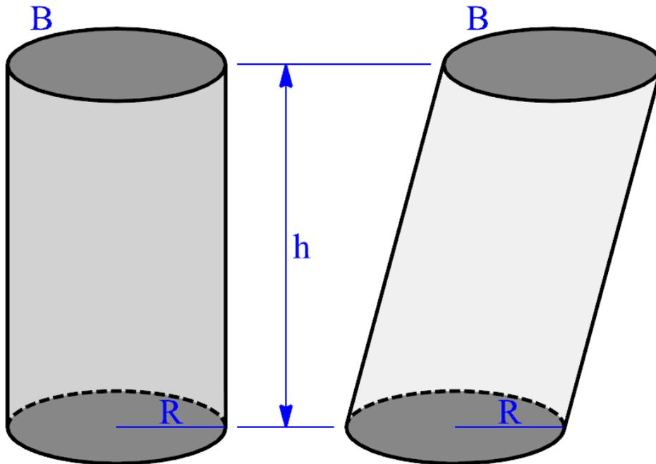
*Figure F-6. A right cylinder and an oblique cylinder.*
