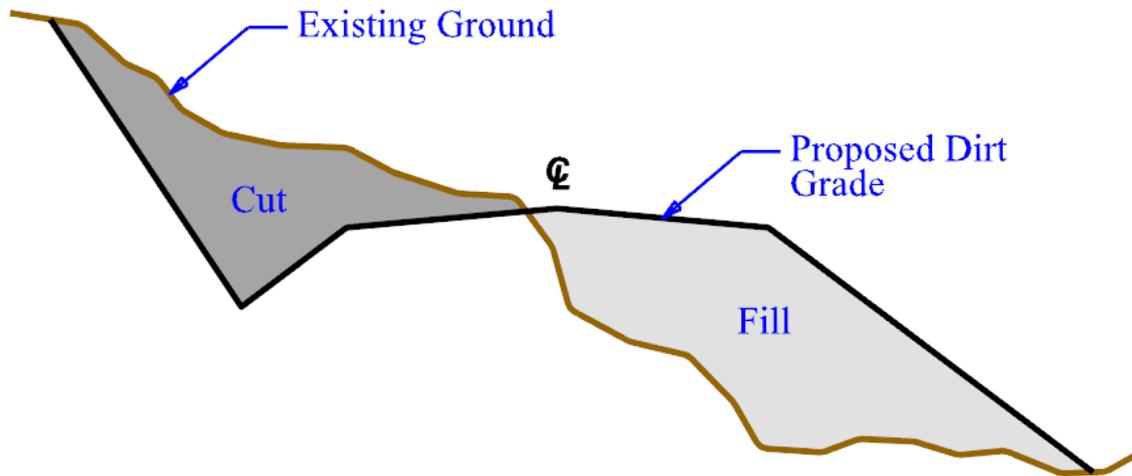
**Figure F-11. Cross-section with cut and fill areas.**
