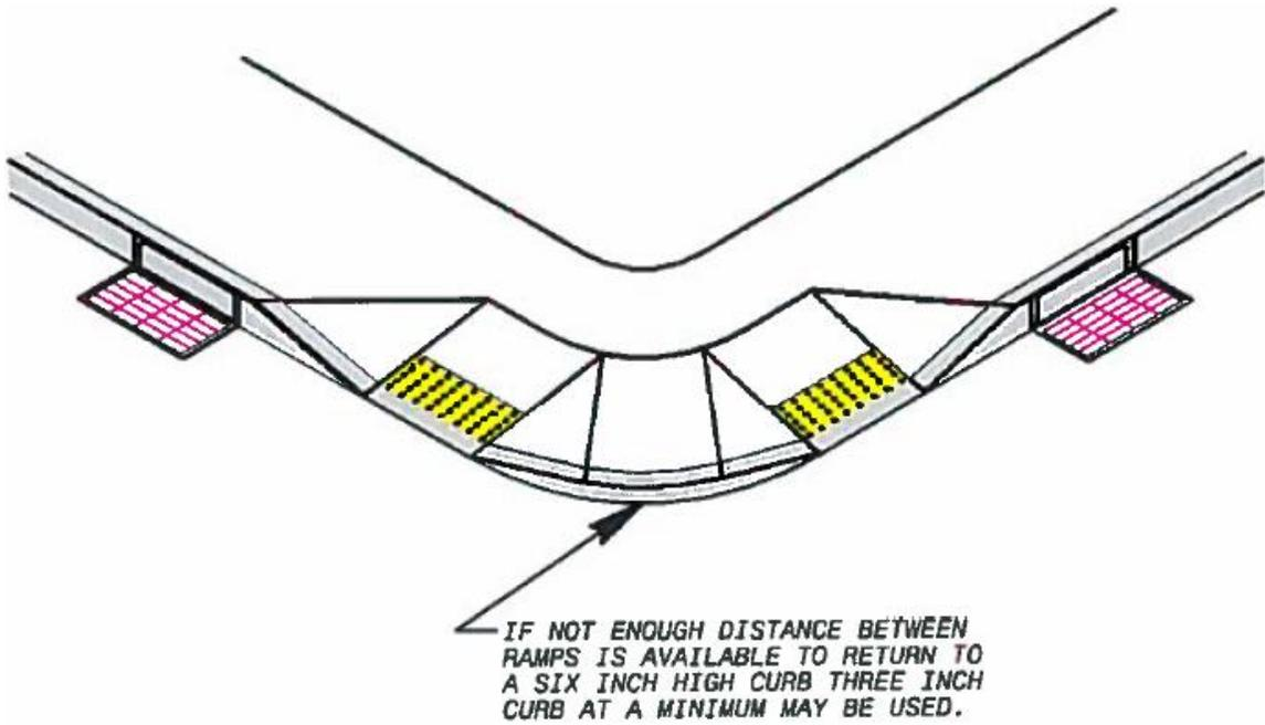
**Figure 32:** Lower Curb Between Ramps
