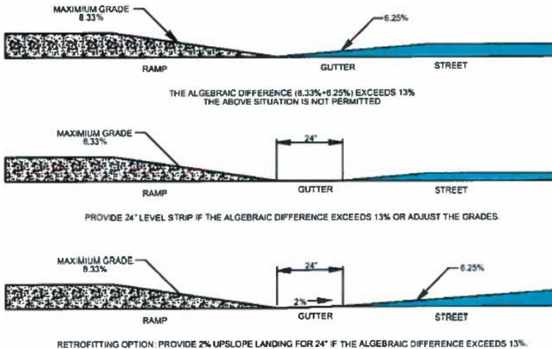
**Figure 16:** Counter Slope
