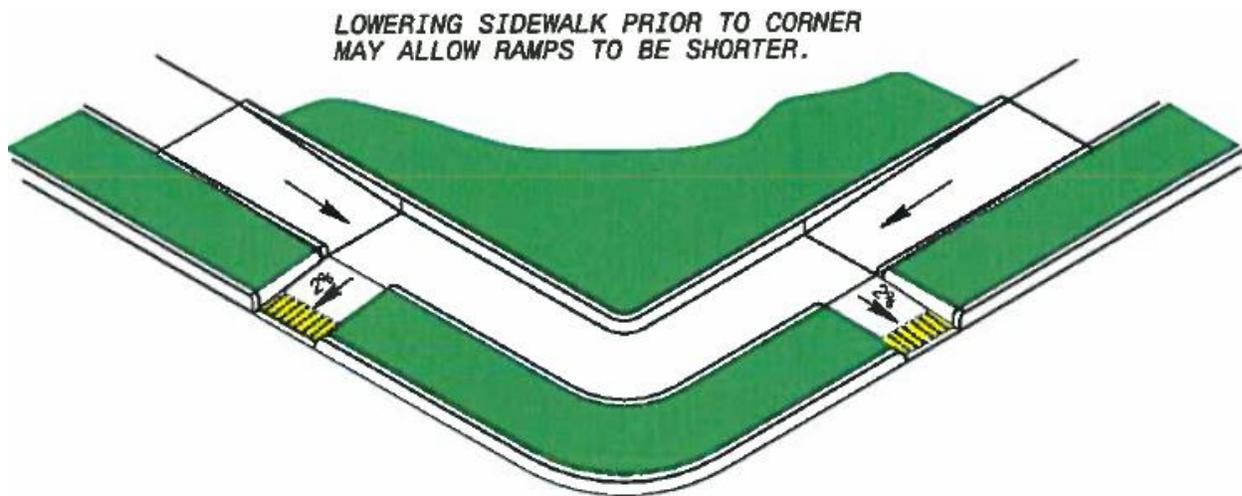
**Figure 29:** Lowering sidewalk in advance of ramp.
