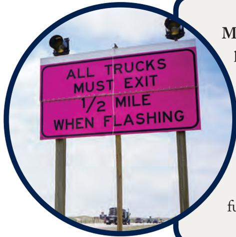
**Maintenance** and **WHP** began an optional procedure for sorting light and high-profile vehicles from passenger vehicles on southbound I-25 at Exit 4 during high wind events.
